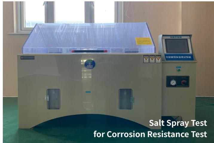
**Salt Spray Test for Corrosion Resistance Test**
