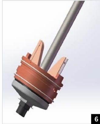
7. Pull the nut washer and remove the seat assembly to clean, inspect, and replace any worn or damaged parts.
