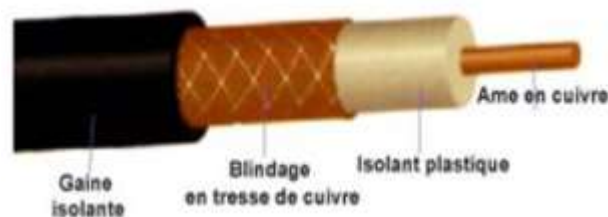
Figure II.9 : Le Câble Coaxial
